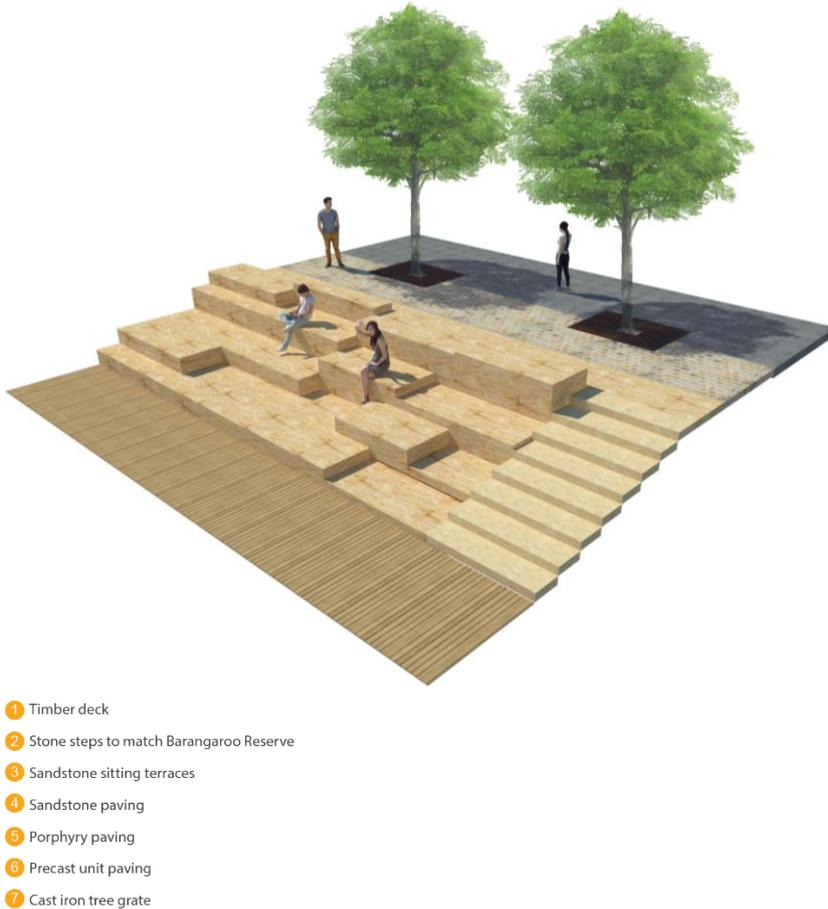
**Figure 18 – Wulugul Walk and Boardwalk paving transition**
